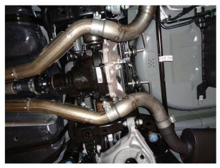
**Step 3.** Begin installation of the new system by attaching both Inlet Pipe Assemblies to the pipes you have just cut. Loosely secure using the supplied 2.50" clamps. Engage the welded hangers to the rubber insulators. Leave all clamps loose until final adjustment. If equiped with valves, be sure to reinstall vavles on new system with wire harness mounting bracket.
