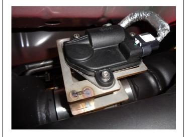
**Step 5.** If your vehicle has valves, re-connect the wiring harness plugs to the Valve motors and wire mounting bracket. If not yet purchased, Valve Kit is part# 10805
